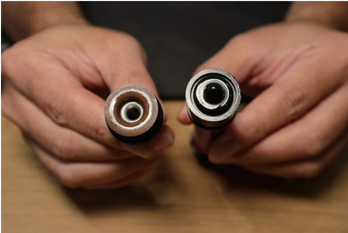
The redesigned enlarged cylinder head (left) and enlarged airbrake piston (right) achieve improved concentrated air pressure.
