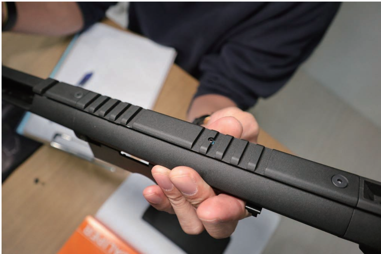
Two-side adjustable hop-up with the original two-side lever as well as the upper screw adjustment.
