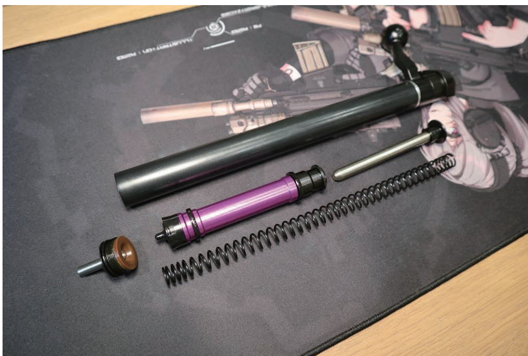
▲ The cylinder; enlarged cylinder head; enlarged O-ring; enlarged piston head; enlarged airbrake piston; 9mm spring; spring guide shown.
