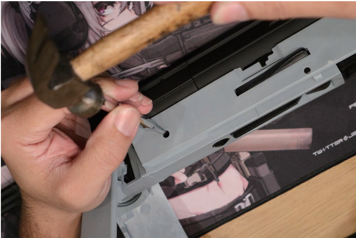
A tool is used to remove the butt stock rocker after securing it the on a jig.
