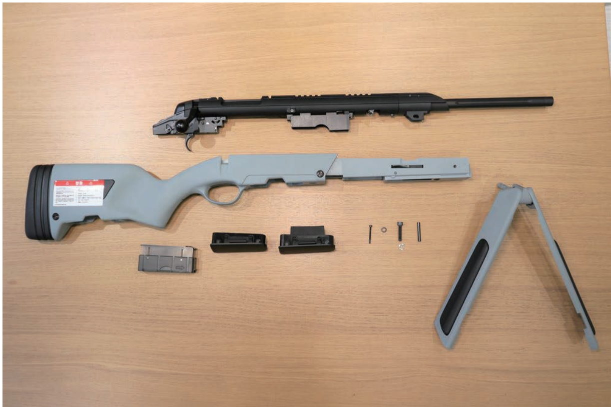
▲ The upper, lower body; magazine; mock hi-capacity magwell; stock takedown screws and pin; stock rocker lock; gun-body washer; and bipod set shown.
